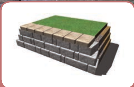
VERTICAL RETAINING WALL
