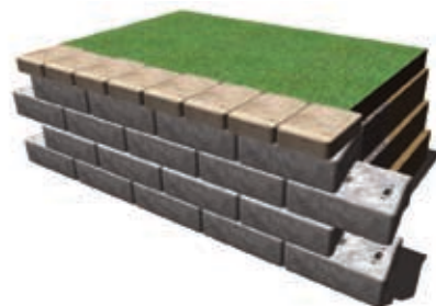
STANDARD RETAINING WALL
